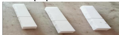
Figure 4.4: 3D printed Impact specimens
