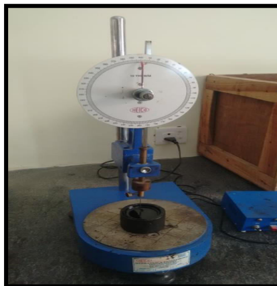
Figure 6.1 Penetration test of Bitumen
