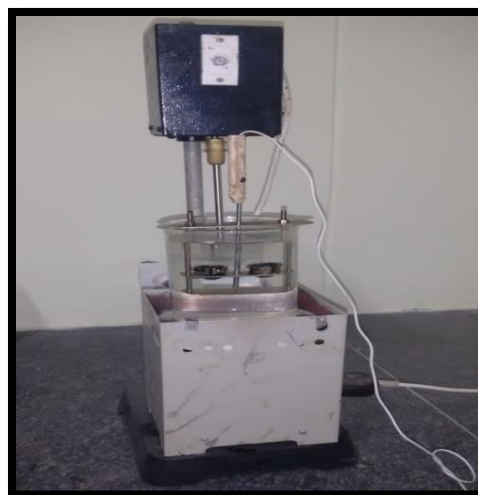
Figure 6.2 Softening point test of Bitumen
