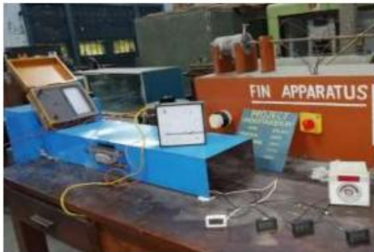
Figure 03: Experimental setup of fins in natural and forced convection analysis.
