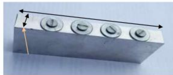
Figure02: Designing of uniform rectangular fin with tapping
