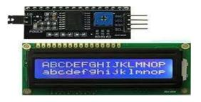
Consequently, each data is sent to LCD in two steps: four higher bits are sent first (that normally would be sent through lines D4-D7),
