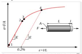
Stress–strain curve showing typical yield behavior  $\ ^{\Box}$  for nonferrous alloys. (Stress  $(\sigma)$  shown as a function of strain  $(\epsilon)$ .)
