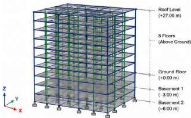
Fig. 5. Three-dimensional analytical model of G+8 residential building developed in STAAD.Pro
