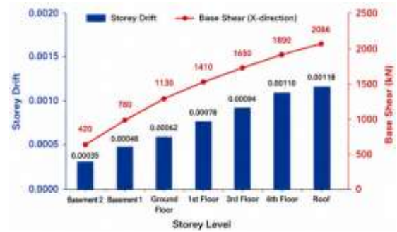
Fig. 9. Comparison of storey drift and base shear response
