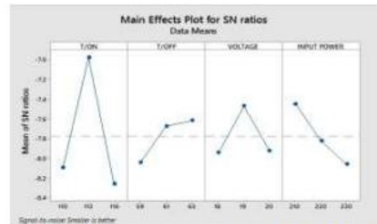
Fig 6. Effect of process parameters on Surface Roughness for S/N ratio
