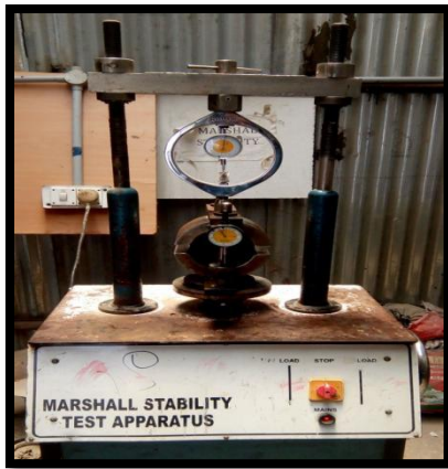
Figure.4 Marshall stability test setup
