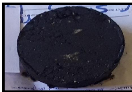
Figure.3 Closer view of Marshall sample
