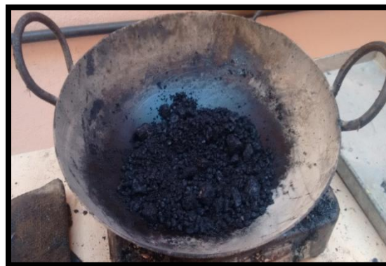
Figure.3 Uniform colour throughout the mix
