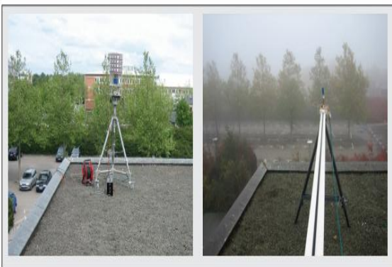
Figure 5. Massive MIMO antenna arrays used for the measurements.
