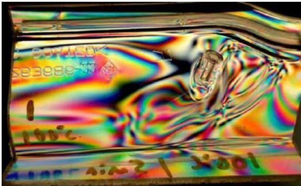
Fig. 3 Residual stress inside the plastic lens. (Source: Elsevier Ltd., 2019).
