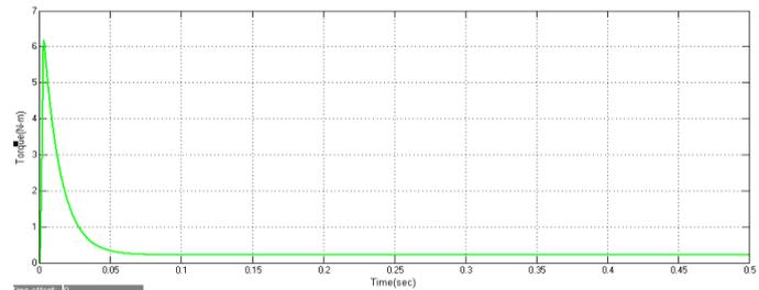
Fig.12 BLDC Motor Drive Torque Characteristics of Proposed Converter
