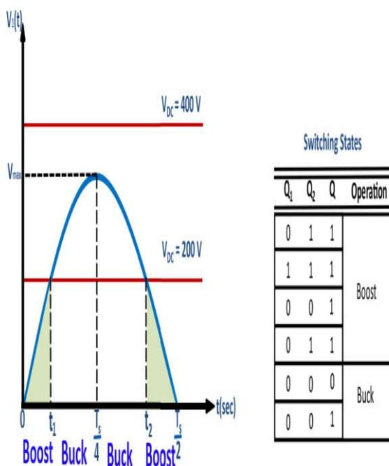
Fig. 2: Rectified input voltage waveform with different possible operating modes and switching states
