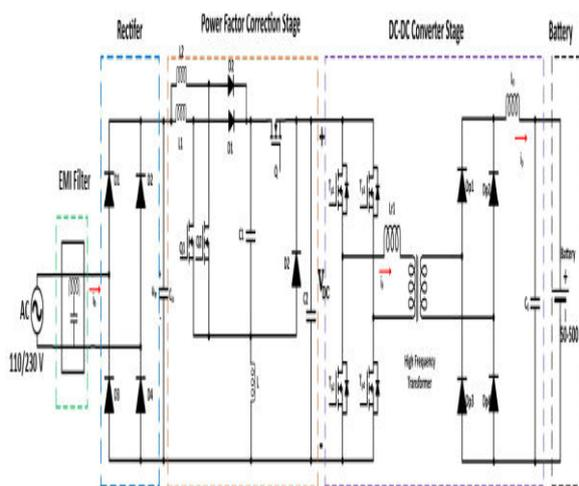
Fig.1: Proposed Interleaved boost cascaded-by buck PFC converter based on-board battery charger. The above circuit shown in Fig.1 is schematic of two stage on-board battery charger. It consists of a power factor correction converter in two-switch topology configuration and an isolated DC-DC converter. The proposed PFC converter consists of a cascaded combination of the interleaved boost
