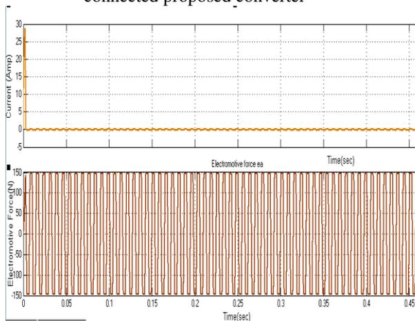
Fig.10 BLDC Motor Drive Stator Current Characteristics of Proposed Converter
