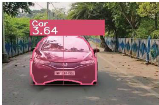
Fig. 6. Average distance estimation using both MiDAS and Mask RCNN (front view)
