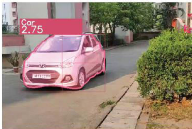
Fig. 7. Average distance estimation using both MiDAS and Mask RCNN (side view).
