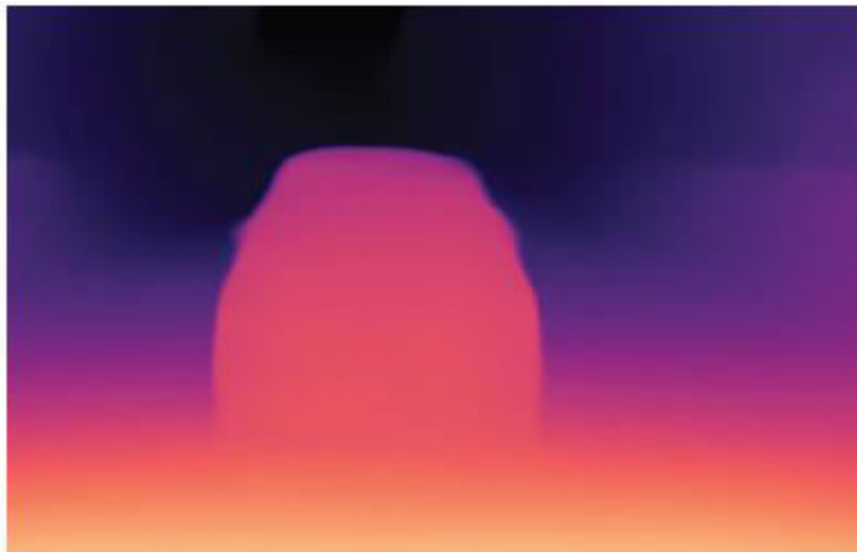
Fig. 4. Depth map from the output of MiDAS for the front facing car
