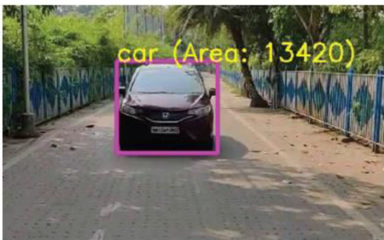
Fig. 2. Object detection with bounding box and associated area (front view)
