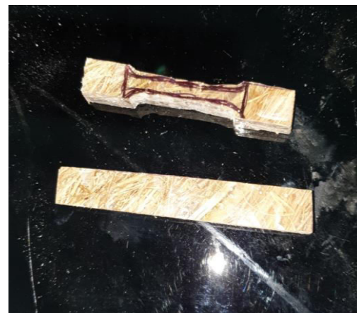
Fig-7: Specimen for tensile and bending stress.
