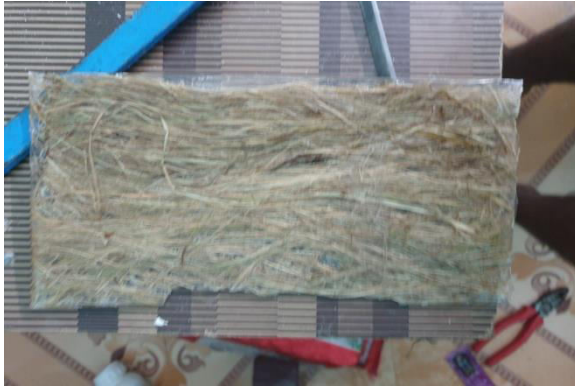
Fig-3: fiber made according to the jute orientation
