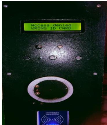
Fig 9: Figure Showing “Access denied WRONG ID CARD” when a wrong (Unauthorized) RFID Card is placed.
