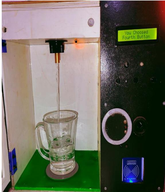
Fig 8: Figure showing the dispensing of water when master card is placed and any of the button is pressed.
