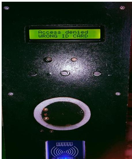
Fig 6:Figure showing the message on LCD display as: “Access denied WRONG ID CARD”, when wrong(unauthorized) card is placed.
