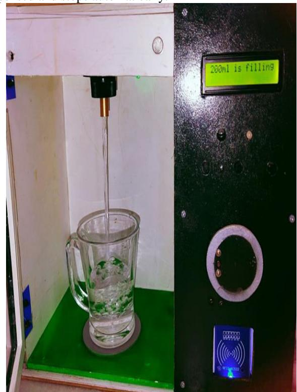
Fig 7:Figure showing the dispensing of water when an authorized card is placed and any of the button is pressed.
