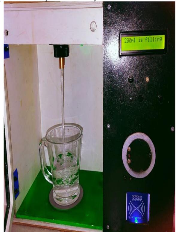
Fig 7Figure showing the dispensing of water when an authorized card is placed and any of the button is pressed.
