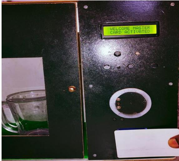
Fig 5:Figure showing the message on LCD display as: “WELCOME MASTER CARD ACTIVATED”, when master card is placed.
