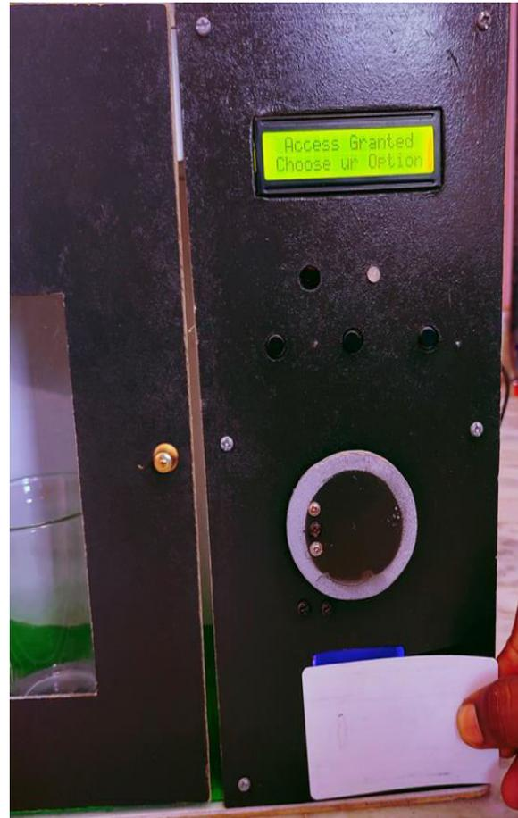
Fig 4:Figure showing the message on LCD display as: “Access Granted Choose Your Option”, when an authorized card is placed.
