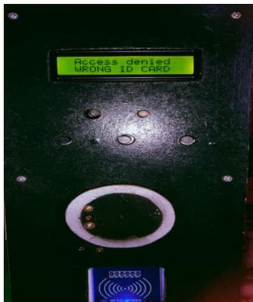
Fig 9: Figure Showing “Access denied WRONG ID CARD” when a wrong (Unauthorized) RFID Card is placed.
